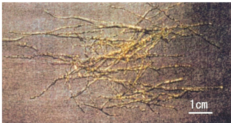
Figure 4 A view of CA-Ta fiber pyrolyzed under \text{NH}_3 at 1400^\circ\text{C} . [Color figure can be viewed in the online issue, which is available at www.interscience.wiley.com .]
